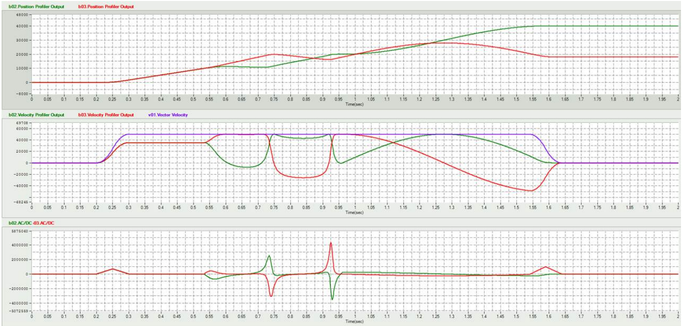
Figure 4-96 Example of Polynomial Function Motion within EAS Application
